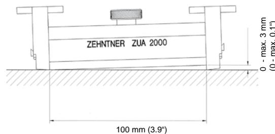
Illustration of a layer with steadily changing thickness (wedge-shaped application)
